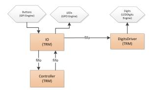
You may wonder why there is a separate component for the 7-digit display. The reason is that controlling the 7-digit display, on a first glance, is not so trivial, so we solved it with a little software loop being implemented on TRM.
