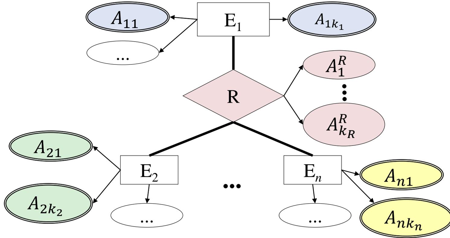
$$R: \left\{ \underbrace{[A_{11}, \dots, A_{1k_1}]}_{\text{Schlüssel } E_1}, \underbrace{[A_{21}, \dots, A_{2k_2}]}_{\text{Schlüssel } E_2}, \dots, \underbrace{[A_{n1}, \dots, A_{nk_n}]}_{\text{Schlüssel } E_n}, \underbrace{[A_1^R, \dots, A_{k_R}^R]}_{\text{Attribute von } R} \right\}$$
