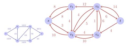
Rest networks provide the same kind of properties as flow networks with the exception of permitting antiparallel capacity-edges
