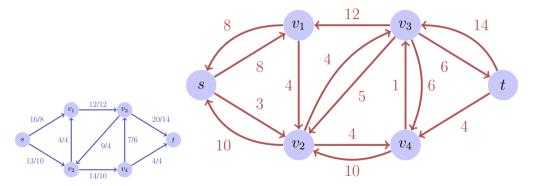
Rest networks provide the same kind of properties as flow networks with the exception of permitting antiparallel edges
