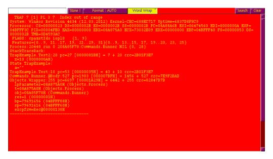
The trap output can be used to diagnose the history of a trap. Inspection of the trap is also
