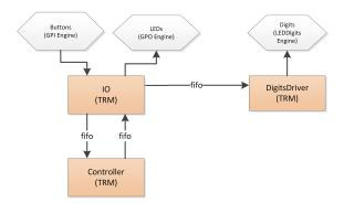
You may wonder why there is a separate component for the 7-digit display. The reason is that controlling the 7-digit display, on a first glance, is not so trivial, so we solved it with a little software loop being implemented on TRM.
